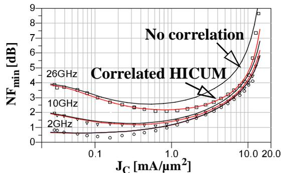
Fig. 5.  $NF_{\min}$  vs.  $J_C$  for SiGe HBTs, symbols: meas., lines: sim.
