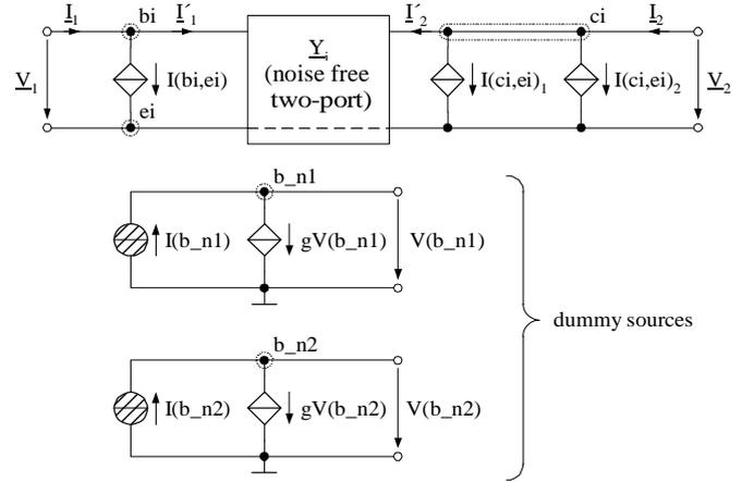
Fig. 3. Realization of correlation in compact models from a system theory perspective.
