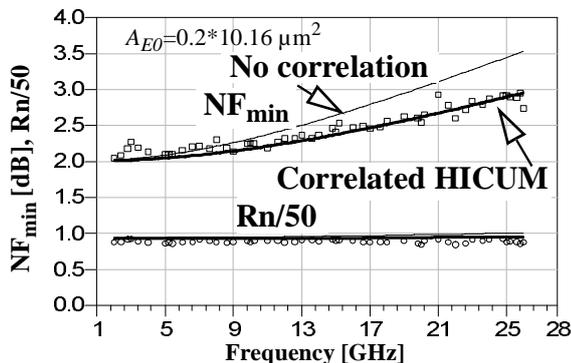
Fig. 6.  $NF_{\min}$  and  $R_n/50$  vs frequency at  $J_C=2.74\text{mA}/\mu\text{m}^2$ ,  $V_{CE}=1.5$  V, meas., lines: sim.
