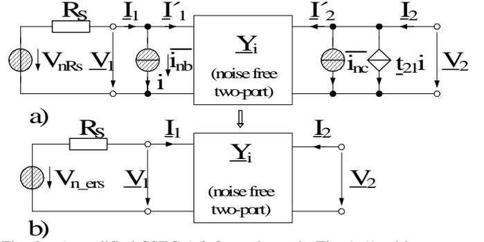
Fig. 2. a) modified SSEC (cf. framed part in Fig. 1 a) with uncorrelated noise sources  $\overline{i_{nb}}$ ,  $\overline{i_{nc}}$  and  $t_{21}i$ , b) SSEC with equivalent noise voltage source  $v_{n_{ers}}$  at the input (usually the input port source).
