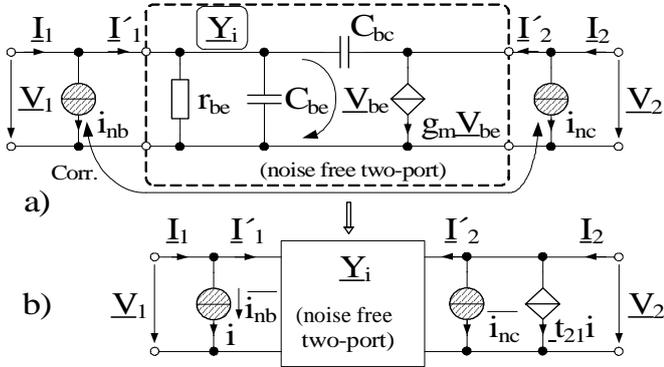
Fig. 1. a) Noise free two-port with small signal equivalent circuit (SSEC) of the internal BJT in the dashed box and correlated noise sources  $i_{nb}$  and  $i_{nc}$ , at the input and output respectively b) SSEC with three modified uncorrelated noise sources. Note that  $i \equiv \overline{i_{nb}}$ .
