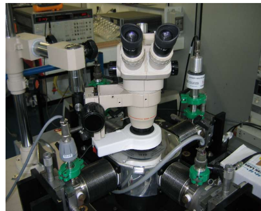
Cryogenic prober for 77K measurements
