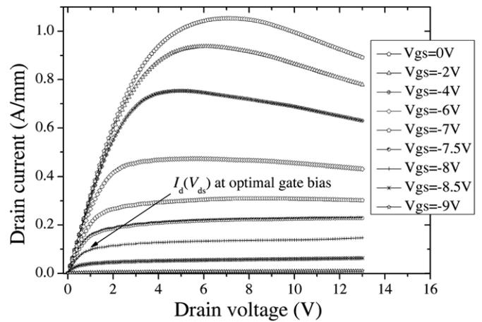
**Figure 3.** Drain current versus drain voltage of device B ( $L_g = 2 \mu\text{m}$ ,  $W_g = 2 \times 50 \mu\text{m}$ ).
