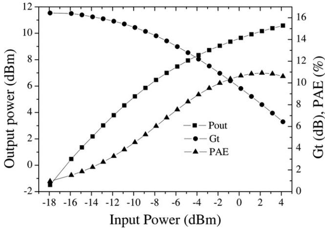
**Figure 4.** Output power versus input power for device A ( $L_g = 2 \mu\text{m}$ ,  $W_g = 2 \times 50 \mu\text{m}$ ) at 4 GHz for  $\Gamma_{\text{Source}} = (0.777; 0.365)$ ,  $\Gamma_{\text{Load}} = (0.829; 0.117)$ ,  $V_{\text{ds}} = 13 \text{ V}$  and  $V_{\text{gs}} = -2 \text{ V}$ .
