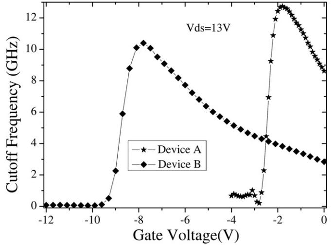
**Figure 6.** Current gain cutoff frequency versus  $V_{\text{gs}}$  for devices A (stars) and B (diamonds) ( $L_g = 2 \mu\text{m}$ ,  $W_g = 2 \times 50 \mu\text{m}$ ).
