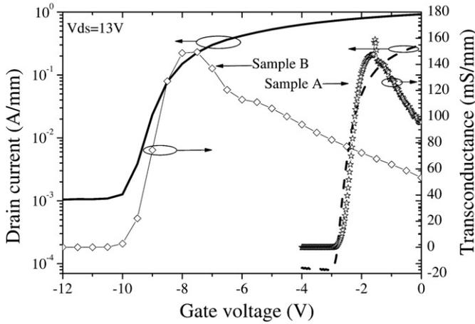
**Figure 1.** Transfer and transconductance characteristics of HFETs ( $L_g = 2 \mu\text{m}$ ,  $W_g = 2 \times 50 \mu\text{m}$ ) for device A (dashed line, stars) and device B (solid line, diamonds).
