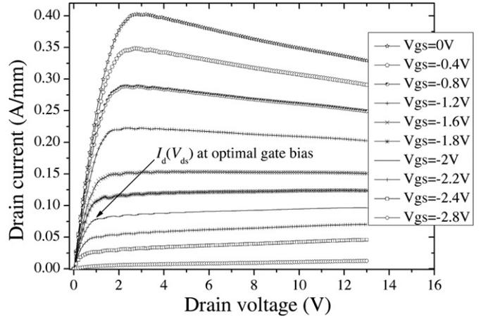
**Figure 2.** Drain current versus drain voltage of device A ( $L_g = 2 \mu\text{m}$ ,  $W_g = 2 \times 50 \mu\text{m}$ ).
