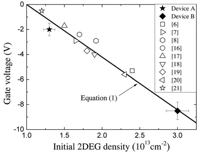
**Figure 7.** Optimal gate voltage dependence on initial 2DEG density of as-grown heterostructures for the fastest short-gate GaN HFETs (open symbols) and long-gate devices A (closed star) and B (closed diamond).
