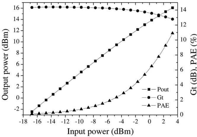
**Figure 5.** Output power versus input power for device B ( $L_g = 2 \mu\text{m}$ ,  $W_g = 2 \times 50 \mu\text{m}$ ) at 4 GHz for  $\Gamma_{\text{Source}} = (0.685; 0.500)$ ,  $\Gamma_{\text{Load}} = (0.797; 0.195)$ ,  $V_{\text{ds}} = 13 \text{ V}$  and  $V_{\text{gs}} = -8 \text{ V}$ .
