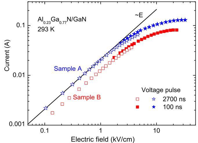
**Figure 3.** Measured dependence of current on electric field for passivated sample A (stars, channel length  $6 \mu\text{m}$ ) and unpassivated sample B (squares,  $12 \mu\text{m}$ ). Voltage pulse duration is  $2.7 \mu\text{s}$  (open symbols) and 100 ns (closed symbols). Solid line represents ohmic behaviour for sample A.
