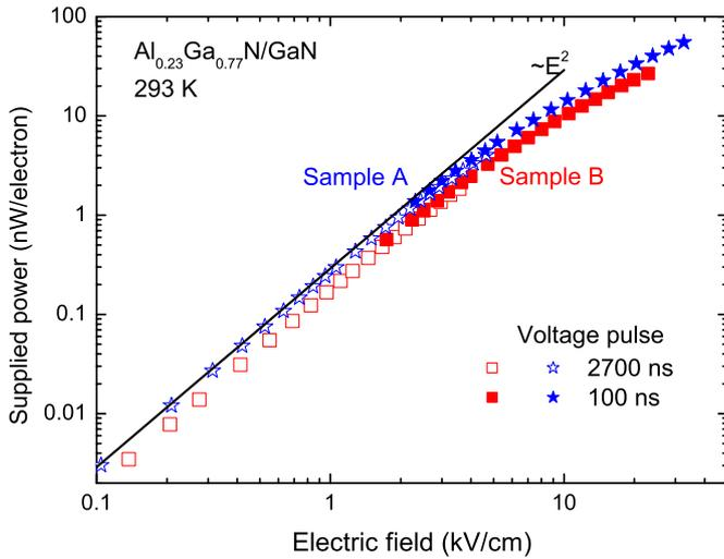
**Figure 5.** Dependence of supplied power per electron on electric field for passivated sample A (stars) and unpassivated sample B (squares). Voltage pulse duration is  $2.7 \mu\text{s}$  (open symbols) and 100 ns (closed symbols).
