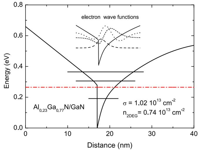
**Figure 1.** Dependence on distance perpendicular to channel plane of conduction band edge energy (solid line). Fermi energy is represented by dashed-dotted line, and electron energy levels for three lowest subbands are represented by horizontal bars. Envelope wave functions for three lowest subbands are given in the inset.
