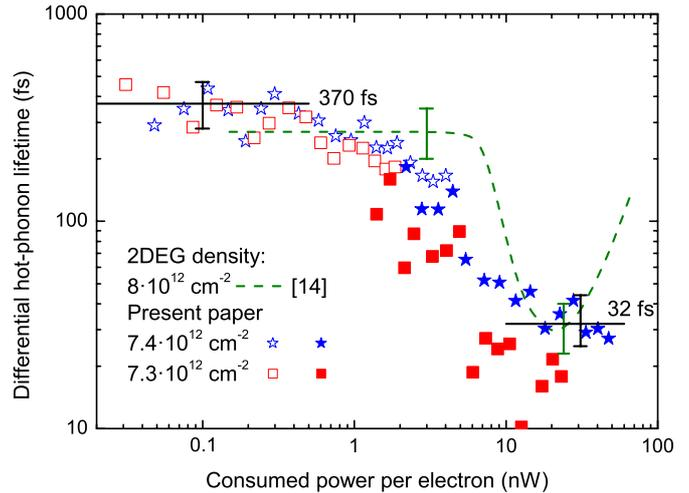
**Figure 8.** Differential hot-phonon lifetime for  $Al_{0.23}Ga_{0.77}N/GaN$  2DEG channels: passivated sample A (stars) and unpassivated sample B (squares). Open symbols assume  $T_b = T_0$ , closed symbols take into account the power-dependent bath temperature (dashed line in figure 6). Dashed curve illustrates the experimental data for  $AlInN/AlN/GaN$  [14]. Black solid lines stand for 370 fs and 32 fs.
