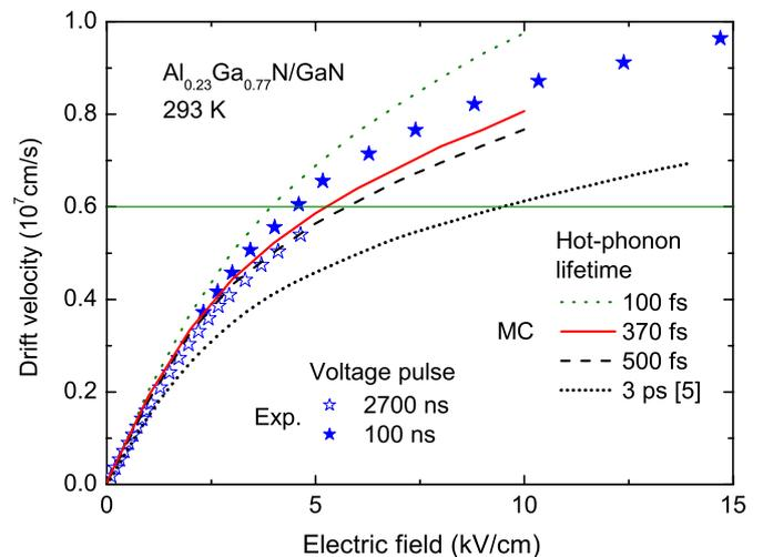
**Figure 4.** Dependence of drift velocity on electric field. Stars stand for estimated values from experiment for passivated sample A. Lines show Monte Carlo simulation for hot-phonon lifetime: 100 fs (dots), 370 fs (solid line), 500 fs (dashes) and 3 ps (short dots [5]).
