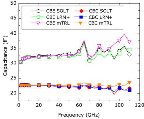
Fig. 4. Extracted junction capacitances  $C_{BE}$  and  $C_{BC}$  of a test HBT for  $V_C=0V$  with respect to three probe-tip calibrations. Results are de-embedded from the Complete-Open and Complete-Short dummies.
