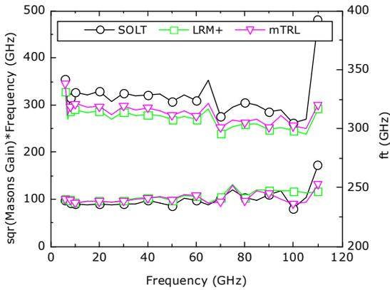
Fig. 5.  $f_{MAX}$  and  $f_T$  of a test transistor calculated at 20 GHz for different probe-tip calibration methods. Results are de-embedded from the Complete-Open and Complete-Short dummies.
