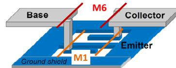
Fig. 1. Location of the measured reference plane after the de-embedding from Pad-Open and Pad-Short (M6) and Complete-Open and Complete-Short (M1).
