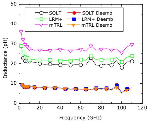
Fig. 3. Inductance  $L1$  of the Complete-Short extracted with respect to different probe-tip calibrations as well as probe-tip calibration follow by de-embedding from the Pad-Open and Pad-Short.  $L2$  exhibits similar behavior
