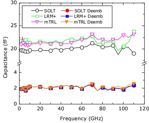
Fig. 2. Capacitance  $C1$  of the Complete-Open extracted with respect to different probe-tip calibrations as well as probe-tip calibration follow by the de-embedding from the Pad-Open.  $C2$  exhibits similar behavior.
