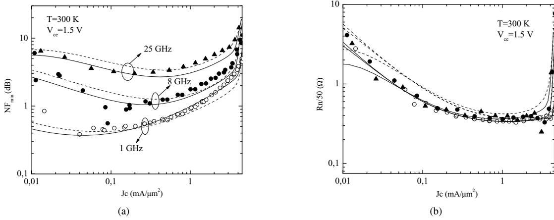
Fig. 5. Minimum noise figure ( $NF_{min}$ ) (a) and noise resistance ( $R_n$ ) (b): solid lines hydrodynamic, dashed lines drift-diffusion model results. Open circles, closed circles, and closed triangles represent the experimental values correspondingly at 1 GHz, 8 GHz and 25 GHz.
