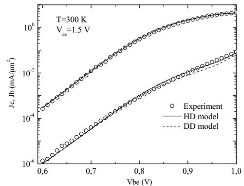
Fig. 1. Collector ( $J_c$ ) and base ( $J_b$ ) current densities: solid lines hydrodynamic and dashed lines drift-diffusion model results. Open circles represent the experimental values.
