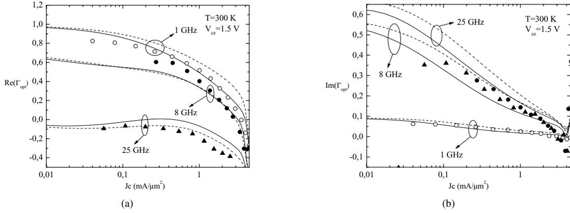
Fig. 4. Real part (a) and imaginary part (b) of the optimum reflection coefficient  $\Gamma_{opt}$ : solid lines hydrodynamic, dashed lines drift-diffusion model results. Open circles, closed circles, and closed triangles represent the experimental values correspondingly at 1 GHz, 8 GHz and 25 GHz.
