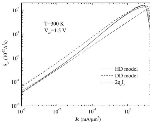
Fig. 6. Spectral intensity of the collector current fluctuations: solid lines hydrodynamic model and dashed lines drift-diffusion model results (black for 1 GHz and gray for 8 GHz). Dotted line—shot noise due to the collector current ( $2q_e I_c$ ).
