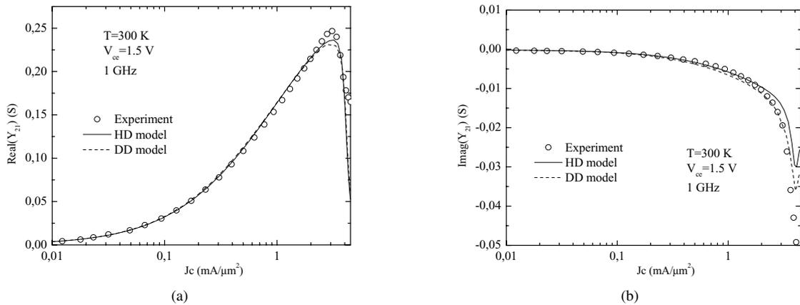
Fig. 3. Real (a) and imaginary part (b) of  $Y_{21}$ : solid lines hydrodynamic and dashed lines drift-diffusion results. Open circles represent the experimental values.
