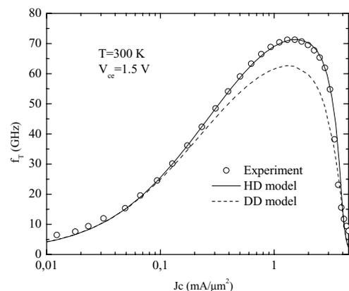
Fig. 2. Cutoff frequency ( $f_T$ ): solid lines hydrodynamic, dashed lines drift-diffusion model results. Open circles represent the experimental values.
