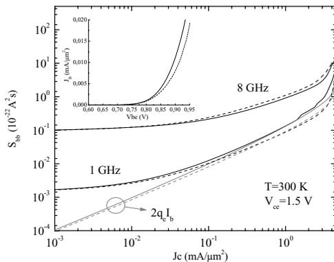
Fig. 7. Spectral intensity of the base current fluctuations: solid lines hydrodynamic model and dashed lines drift-diffusion model results. Gray color represents the shot noise due to the base current ( $2q_e I_b$ ). The base current is shown in the inset of the figure.
