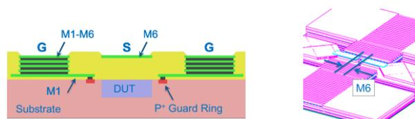
Fig. 1 Design of the DUT RF pad (a) and the location of the measurement plane at metal 6 level M6 (b).
