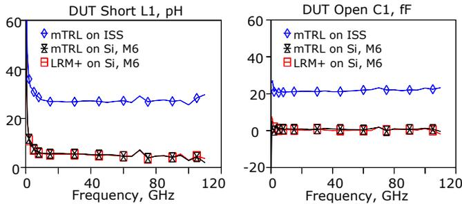
Fig. 6 The inductance L1 of the DUT Short dummy (left) and the capacitance C1 of the DUT Open dummy (right) extracted with respect to the probe-tip mTRL, on-wafer mTRL and on-wafer LRM+ calibration.
