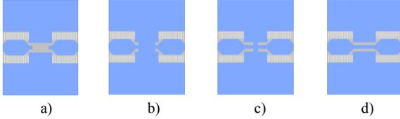
Fig. 2 De-embedding Pad Open (a) Pad Short (b) and calibration Reflect (c), and Thru (d) elements.
