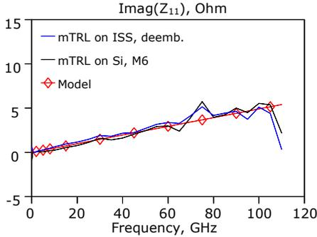
Fig. 5 On-chip Load reactance measured with respect to a probe-tip mTRL followed by the Open-Short de-embedding and the on-wafer mTRL.
