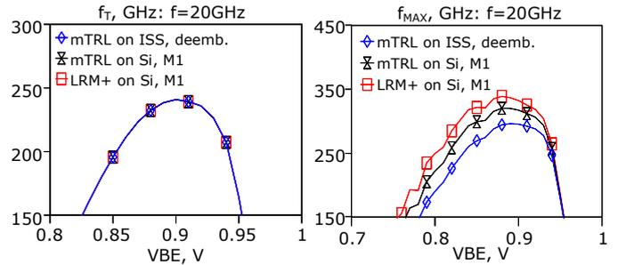
Fig. 8  $f_T$  (left) and  $f_{MAX}$  (right) of the DUT extracted with respect to the probe-tip mTRL followed by the de-embedding, on-wafer mTRL and on-wafer LRM+ calibration (zoomed view).
