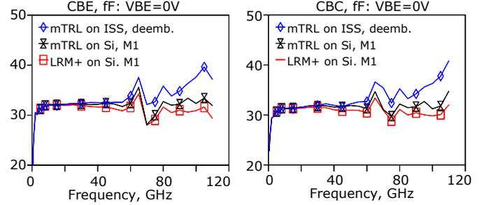
Fig. 7 CBE (left) and CBC (right) of the DUT extracted with respect to the probe-tip mTRL followed by the de-embedding, on-wafer mTRL and on-wafer LRM+ calibration.
