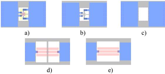
Fig. 3 Design of the DUT (a), the DUT Short (b), the DUT Open (c) the Load (d) and serial Attenuator (e) elements. The load has a single (per measurement port) 50  $\Omega$  N+ salicided poly resistor located at the M1 level. The picture shows the zoomed view of each element.
