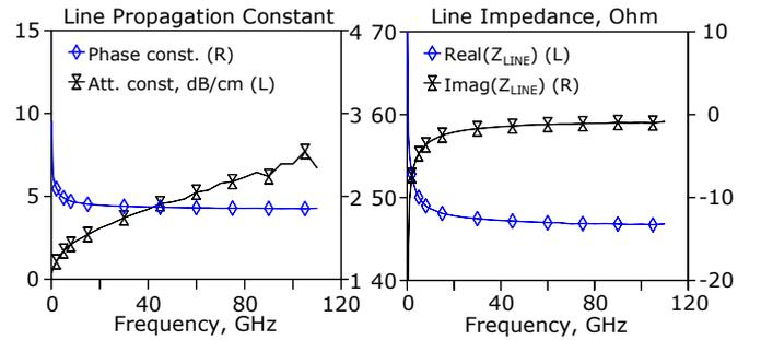
Fig. 4 The relative phase, the attenuation constants (left) and the characteristic impedance  $Z_0$  (right) of the calibration Line.
