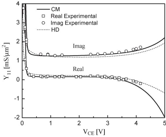
Fig. 5. Real and imaginary parts of  $Y_{11}$  versus CE voltage at 8 GHz. Comparison between (dashed lines) HD model, (symbols) experimental results, and (solid lines) HICUM.
