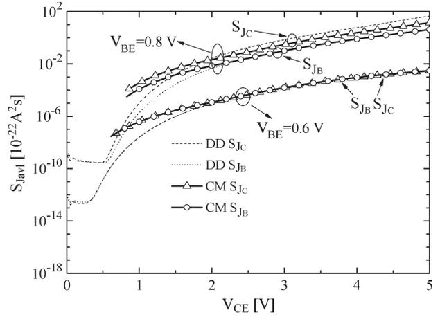
Fig. 14. Collector and base terminal current fluctuations due to II for two different  $V_{BE}$ : Comparison between DD device simulation (dashed lines) and HICUM (solid lines with symbols).
