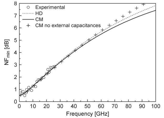
Fig. 11.  $NF_{min}$  versus frequency at  $V_{CE} = 1.0$  V and  $V_{BE} = 0.8$  V. Measured data were obtained with ATN system.
