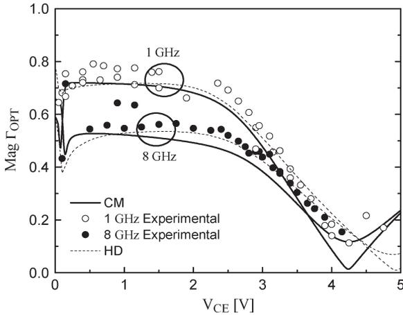
Fig. 9. Magnitude of optimum source reflection coefficient  $\Gamma_{OPT}$  versus CE voltage. (Dashed line) HD simulation results with s.h. and II, (solid line) HICUM, and (scattered line) measurements.
