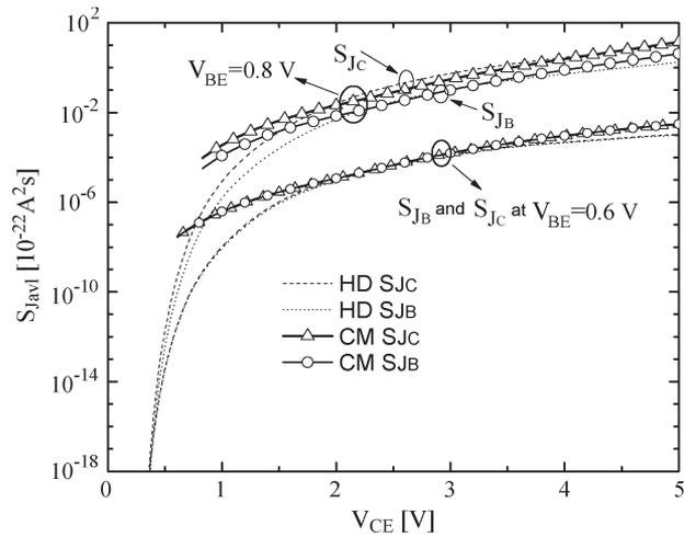
Fig. 15. Collector and base terminal current fluctuations due to II for two different  $V_{BE}$ : Comparison between HD device simulation (dashed lines) and HICUM (solid lines with symbols).
