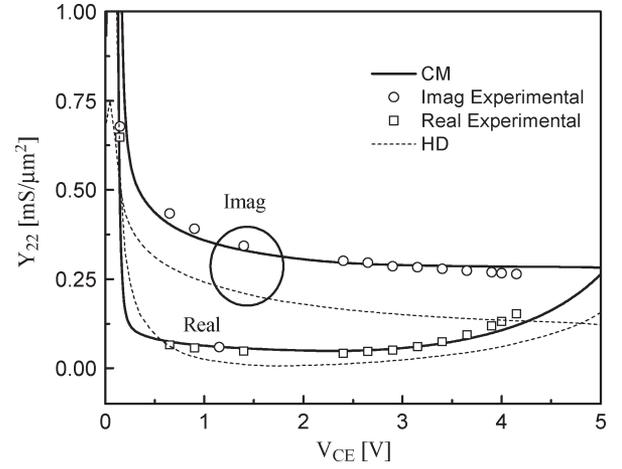
Fig. 7. Real and imaginary parts of  $Y_{22}$  versus CE voltage at 8 GHz. Legend as in Fig. 5.
