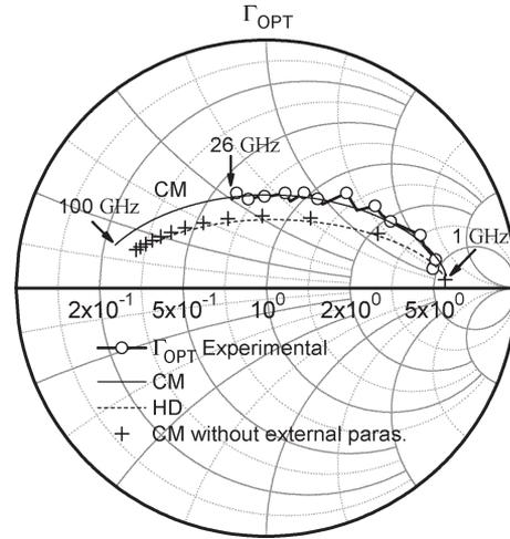
Fig. 12.  $\Gamma_{OPT}$  versus frequency at  $V_{BE} = 0.8$  V. (Dashed line) HD simulation, (solid line) complete HICUM, (crosses) HICUM without external parasitic capacitances and substrate network, and (scattered line with open symbols) measured data.
