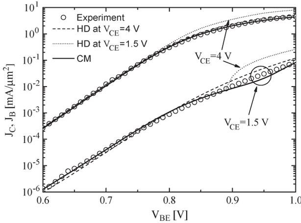
Fig. 1. Forward Gummel characteristics: Comparison between (dashed lines) HD model, (solid lines) HICUM, and (circles) experimental results at  $V_{CE} = 1.5$  V. In addition, HD results are inserted for  $V_{CE} = 4$  V.
