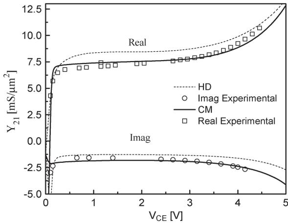
Fig. 6. Real and imaginary parts of  $Y_{21}$  versus CE voltage at 8 GHz. Legend as in Fig. 5.
