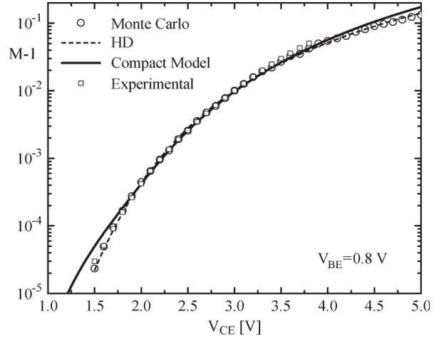
Fig. 3. Avalanche multiplication factor dependence on the applied CE voltage.
