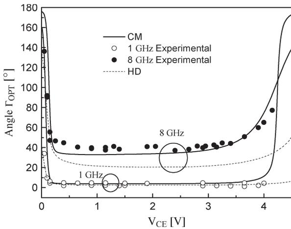
Fig. 10. Phase of optimum source reflection coefficient  $\Gamma_{OPT}$  versus CE voltage. Legend as in Fig. 8.
