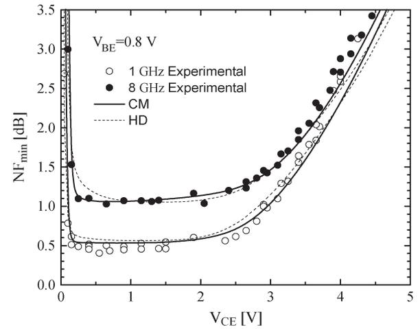
Fig. 8. Minimum noise figure  $NF_{\min}$  versus CE voltage: (Dashed lines) HD simulation results with s.h. and II, (solid lines) HICUM, and measurements at (open circles) 1 GHz and (filled circles) 8 GHz, respectively.
