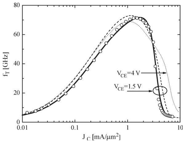
Fig. 2. Transit frequency versus collector current density. Legend as in Fig. 1.
