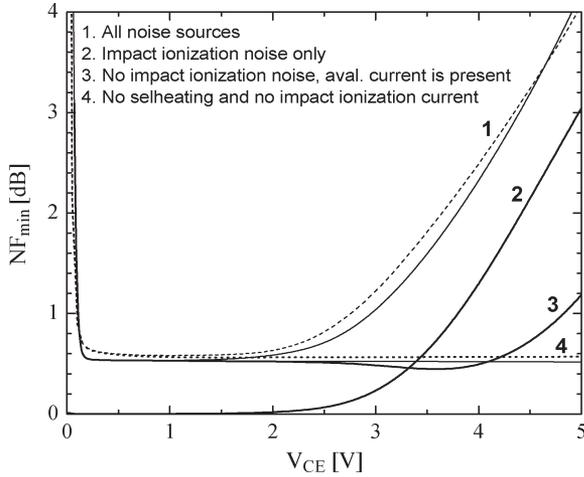
Fig. 13. Resolved noise sources for  $NF_{\min}$  versus  $V_{CE}$  obtained from (solid lines) HICUM simulations at 1 GHz: (Curve 1) Complete model, (curve 2) noise from II only and no s.h., (curve 3) with avalanche effect and multiplication of shot noise but neglecting II noise, and (curve 4) neither II noise nor s.h. In addition, Galene results are inserted for cases 1 and 4.
