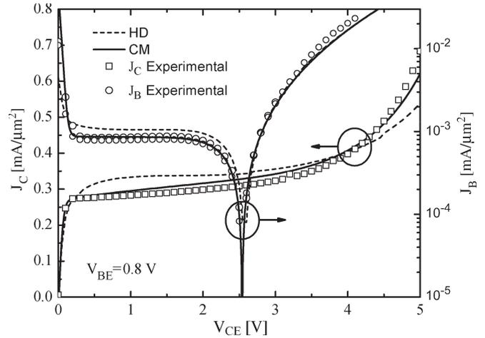
Fig. 4. Base and collector current dependence on CE voltage: (Dashed lines) HD model, (solid lines) HICUM, and (circles) experimental results.
